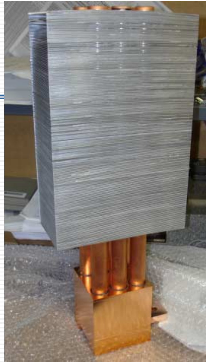
Press pack thyristor cooler using 25.4 mm dia heat pipes.
